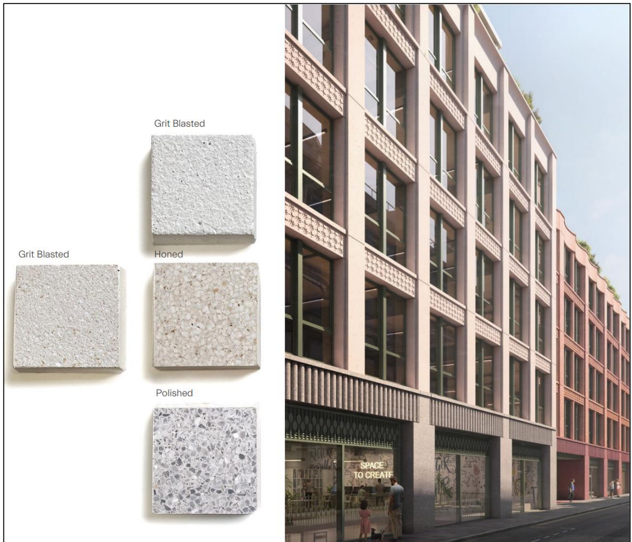
Figure 26: Material Palette of the 'Factory' element to the western side of Epworth Street
